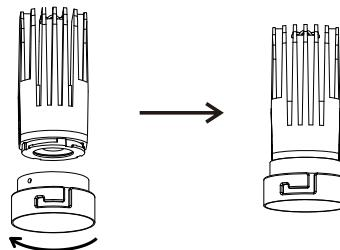
3. Twisting the lighting fixture part appropriately onto the plaster frame.
